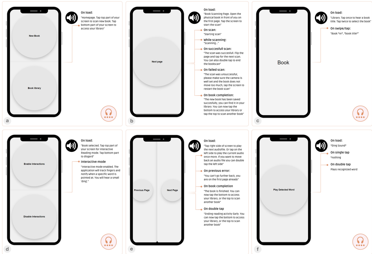
Figure 4: Interaction Design of WordBond: Application User Interfaces and Core User Flow
