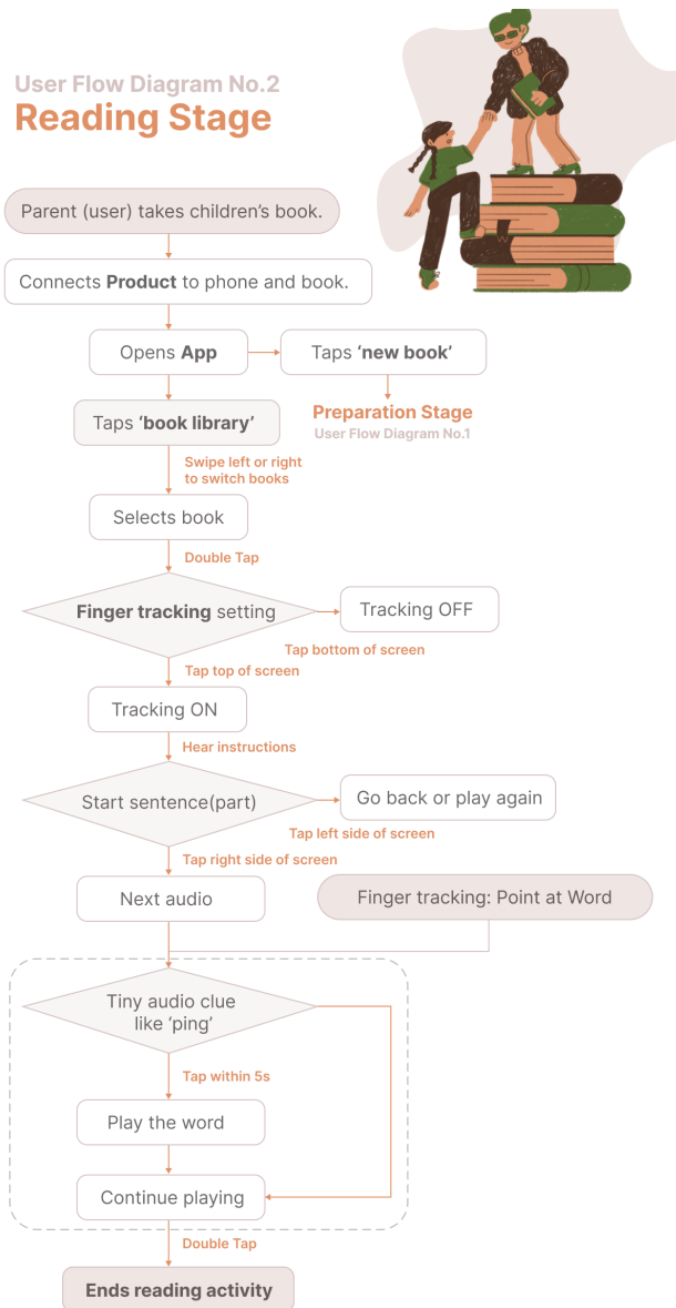
Figure 11: User Flow Diagram 2: Reading Stage.
